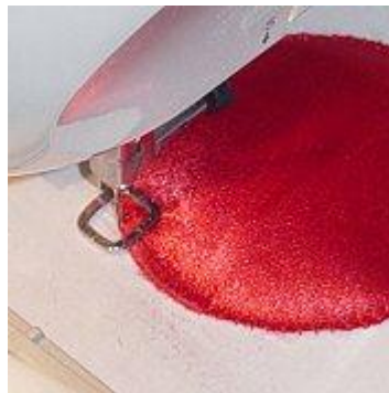
Step 5: Attach hoop to machine and stitch tack down and satin stitch.
